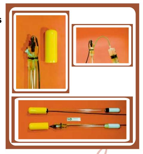
Skye automatic electronic tensiometers are precision made devices for measuring soil moisture pressure or water potential. They measure directly in HectoPascals (or mbar) the suction pressure required to utilise the water in the measured area, and hence the water available to the plant.
